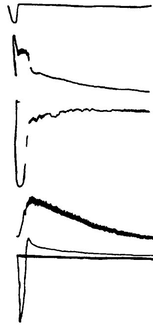
FIG. 2. Oscilloscope traces of the variations in the macroscopic plasma characteristics during the heating and cooling phases. The scan duration is 0.1 \text{ s} .
