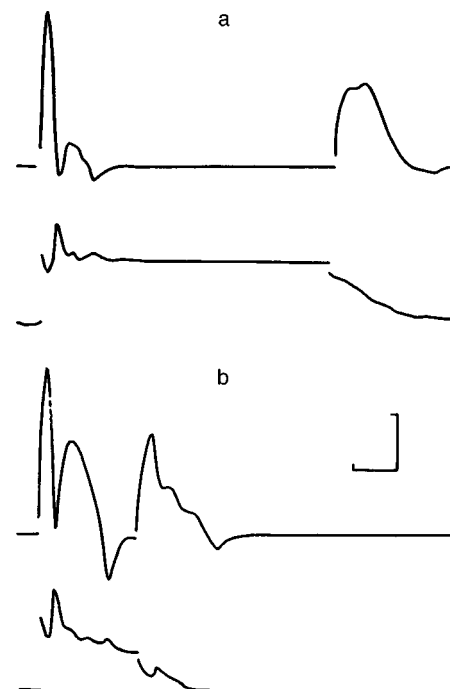
FIG. 3. Oscillograms of the discharge current (upper traces) and residual voltage (lower traces) in the detonation of an aluminum wire of diameter 1 mm and length 30 cm in water: (a) detonation at a discharge voltage of 4 kV; (b) detonation at 5 kV.
