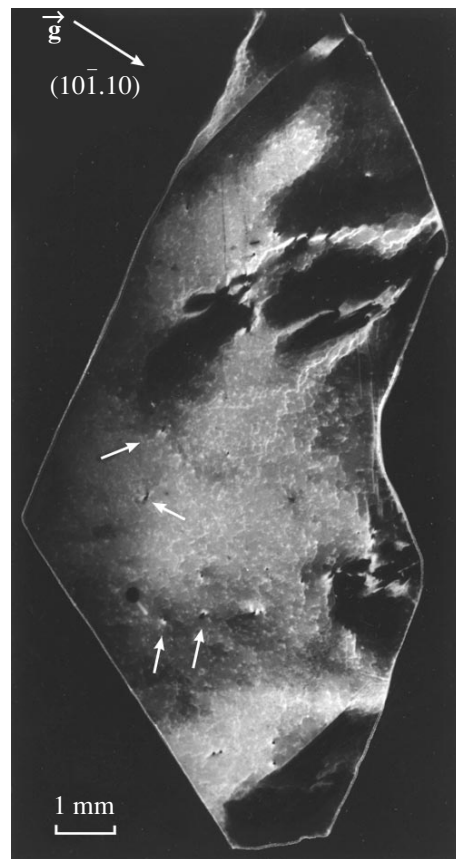
Fig. 4. Double-crystal x-ray topogram of the substrate with an epitaxial layer [ \text{CuK}\alpha radiation, (10\bar{1}.10) reflection]. Defects with a dark core and bright halo are micropipes.
