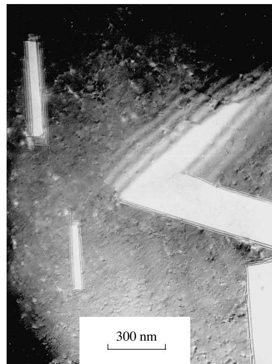
Fig. 2. TEM microphotographs of the \text{TiO}_{1.087} sample (115000x magnification). The extended rectangles are twins; the angle of the twin with broad extinction contours (on the right and slightly above the middle of the figure) is large ( \sim 90^\circ ), and the remaining twins with narrow extinction contours belong to the second family.
