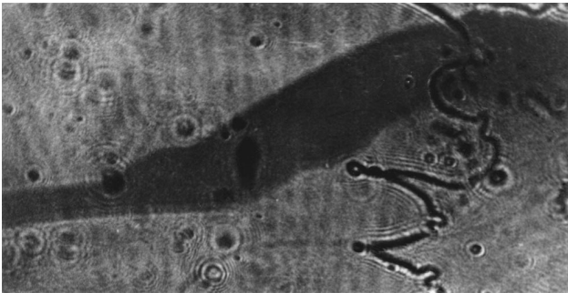
Fig. 2. Double-exposure high-speed photograph of a generated pair of two solitary flexural waves moving in opposite directions and accompanying the antiferromagnetic vortex and antivortex in a domain wall moving at a velocity of 12 km/s in a yttrium orthoferrite plate.
