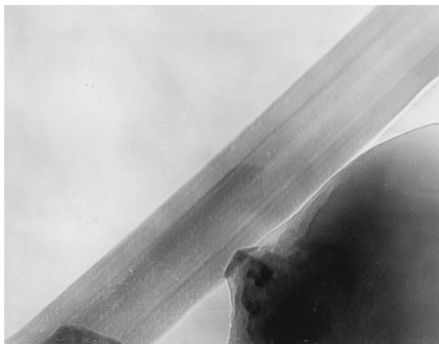
Micrograph of a carbon nanotube prepared from poly(vinyl alcohol) in the \text{H}_2\text{V}_{10}\text{Mo}_2\text{O}_{31} medium.
