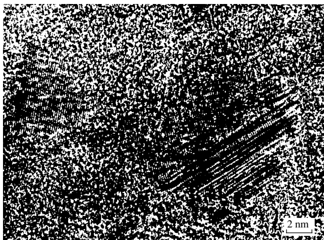
Fig. 7. High-resolution image of the microstructure of the (\text{Ni}_{65}\text{Mo}_{35})_{90}\text{B}_{10} alloy.
