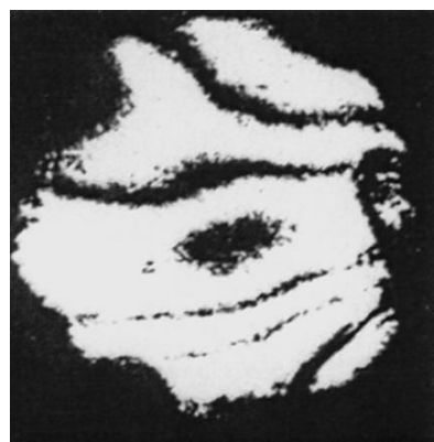
Fig. 2. Interferogram reconstructed from two multiple-exposure holograms in the interferometric correlator.
