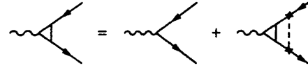
FIG. 2. Electron–electron interaction vertex in which electron–impurity scattering is taken into account in the ladder approximation.
