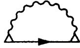
FIG. 1. Diagram of electron self-energy taking into account electron–electron interaction in the first order of perturbation theory.
