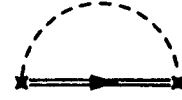
FIG. 3. Diagram of electron self-energy, illustrating renormalization of the impurity collision integral due to electron–electron interaction. The double solid line represents the electron Green's function with due account of electron–electron interaction.
