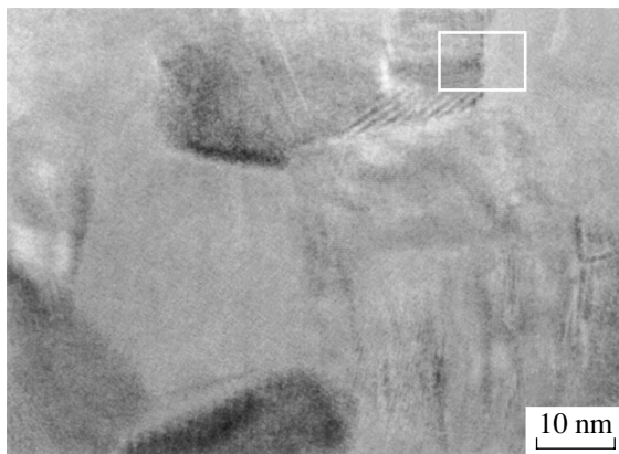
Fig. 5. Microstructure of a Zr_{50}Ti_{16}Cu_{15}Ni_{19} alloy sample obtained after thermal treatment at T = 773 K.
