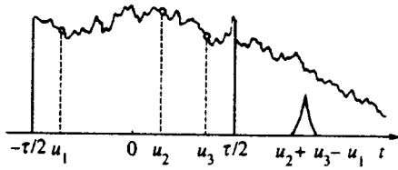
FIG. 2. Time diagram of the excitation of stimulated correlation echo from three noise counts at times u_1 , u_2 , and u_3 .
