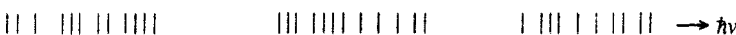
FIG. 6. Spontaneous emission of photons by a molecule with a triplet level exposed to cw laser light (photon bunching).
