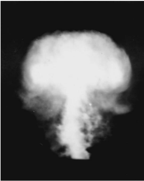
Fig. 4. Mushroomlike plasma cloud produced at \Pi < \Pi_0 and \Delta t_{ej} > \tau_v .
