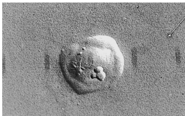
Fig. 4. Microdamages on the anode surface of the NaCl crystal layer in the vicinity of the charge transfer channel.
