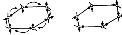
FIG. 3. Fragment of ice lattice containing the shortest cycle of six hydrogen bonds. Protons are shown by closed circles. The arrows depict six sequential proton jumps (creation of a pair of ionic defects on the first jump, subsequent motion of the positive defect along the closed circuit, and its annihilation on the sixth jump). As a result of these six sequential jumps, the left-hand proton configuration transforms to the right-hand one, which is the one closest to it.
