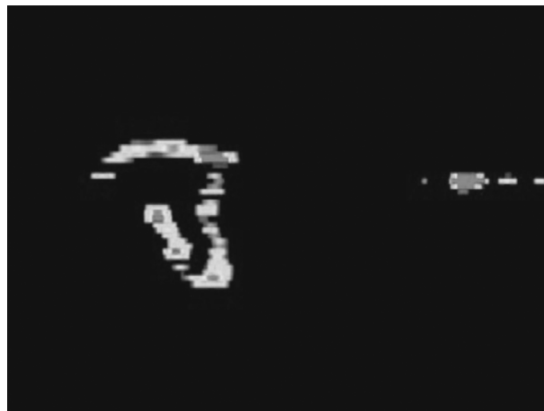
Fig. 4. A beta-alpha coincidence. The electron is from the \beta decay of ^{214}\text{Bi} and the alpha is from the \alpha decay of ^{214}\text{Po} .
