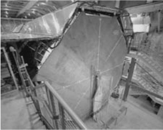
Fig. 2. MINOS Far Detector in the Soudan mine (downstream part of the second supermodule).
