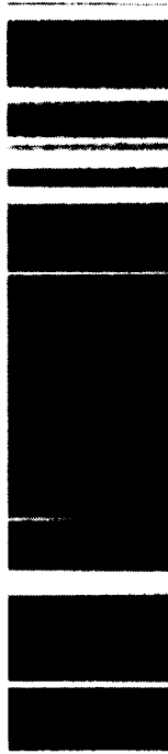
FIG. 2. Typical example of the simplest information-compressed structure of an edge laser speckle pattern (in the far field when the cutting area of the blade is illuminated by a small aperture focused Gaussian argon laser beam).
