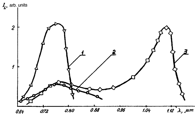
FIG. 1. Photoluminescence spectra of undoped zinc telluride epitaxial films at 77 K: 1 — initial epitaxial film; 2 — epitaxial film after heat treatment in saturated vapor or molten zinc; 3 — epitaxial film after heat treatment in saturated tellurium vapor.
