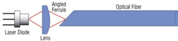
Figure 3.1: Laser diode's emitted light focused into an angled ferrule of a fiber
