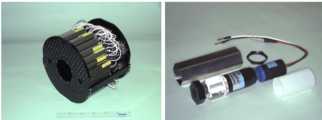
Figure 2.3: On the left a photograph of the BBC array, and on the right a single PMT and radiator element.
