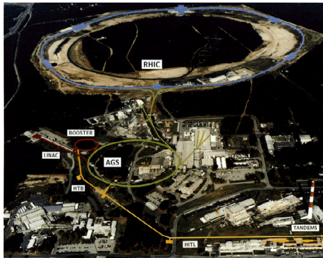
Figure 2.1: The RHIC facility as seen from the air. The circumference of the main RHIC ring is 2.4 miles.
