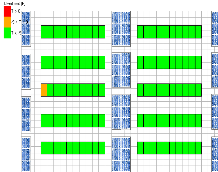
Figure 23: Kool-IT Overheat Plot at 12kW
