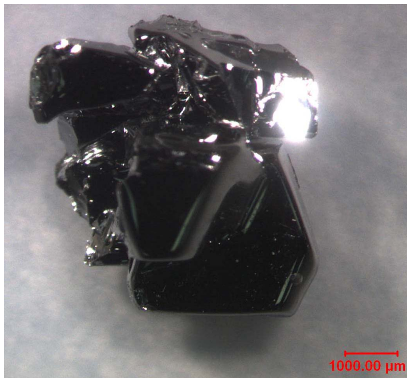
Figure 6.3 The modified Flux method for FeSb 2 single crystal preparation and the single crystal grown by this method
