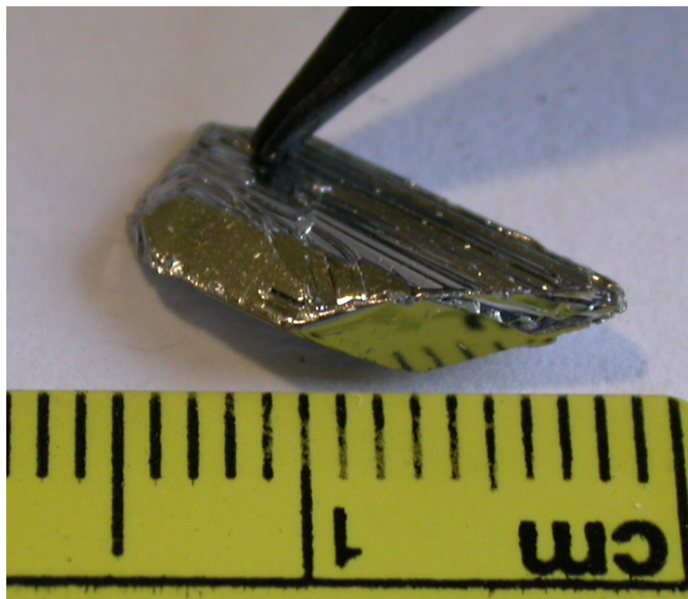
Figure 6.2 The traditional Flux method for FeSb 2 single crystal preparation and the single crystal grown by this method.
