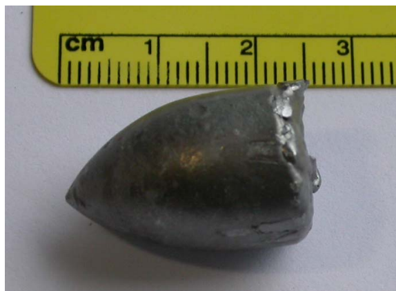
Figure 2.2 An example of quenched filled skutterudite ingot
