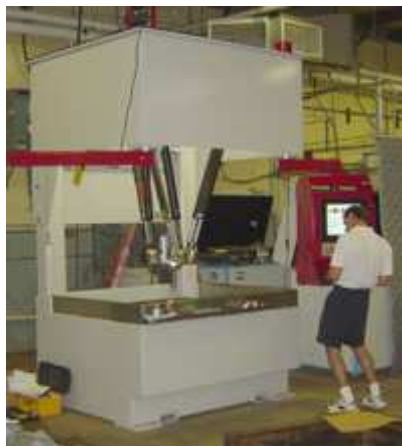
Figure 1.2: 5 Axis Water-Jet Cutting System. Source: courtesy of Mikrolar Inc.( http://mikrolar.com/waterjet.html )
