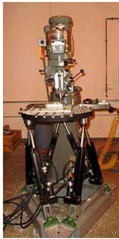
Figure 1.1: A parallel manipulator being used in manufacturing process. Source: courtesy of Mikrolar Inc.( http://mikrolar.com/industrial.html )
