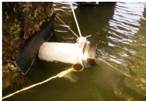
Figure 3. In situ filtration chamber, with plastic bag attached to it, is held onto the pillar of Ponquogue Bridge by rope. Tube for sampling can be seen on top of the PVC pipe.
