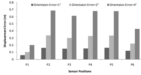
Figure 5-18: Illustration of displacement error for different orientation errors.
