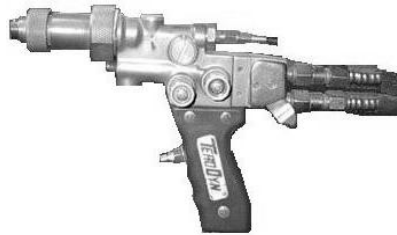
Figure 10: TheroDyn Flame Spray Torch used for the work described in this manuscript
