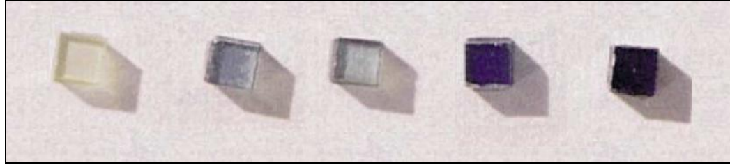
Figure 5: Single Crystals of Titanium Dioxide show different colors as a function of annealing temperature and surrounding atmosphere. Adapted from [43]
