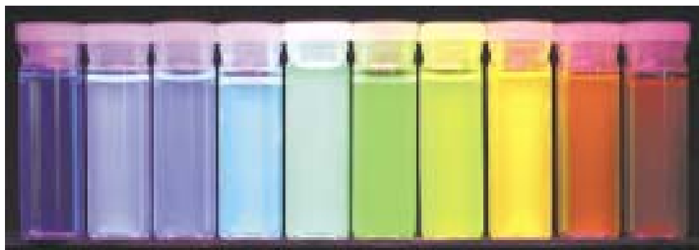
Figure 5-7. Ten distinguishable emission colors of CdSe QDs capped with ZnS 92 (Figure adapted from Ref. 92)
