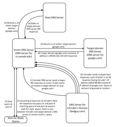
Figure 5.1: Architecture of PRISM model of Kaminsky DNS attack.
