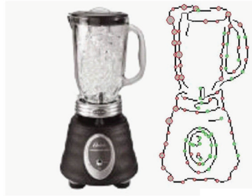
(a) Images with corresponding edge images. The edge images have the random points highlighted. The green points are the ones with no good match.
