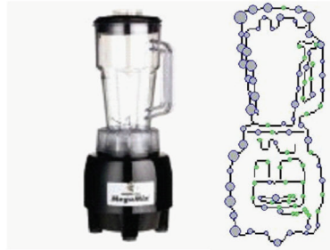
(a) Images with corresponding edge images. The edge images have the random points highlighted. The green points are the ones with no good match.
