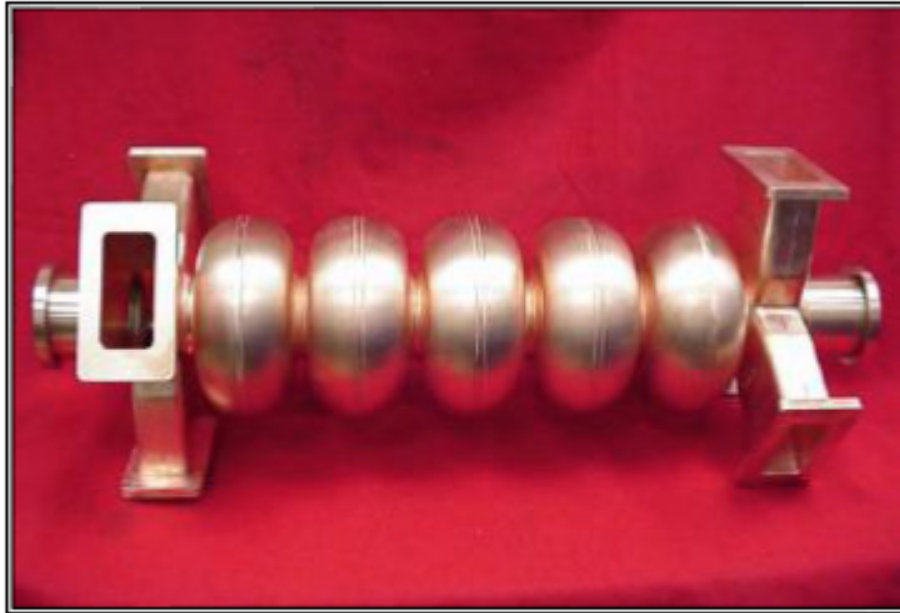
Figure 1.11: Waveguide HOM dampers on a CEBAF cavity at Jefferson Lab.
