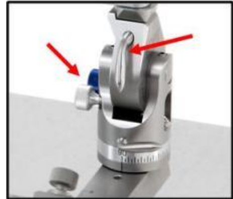
Figure 4: Model 900 Lever Arm Base In terms of mechanical movement reproducibility, one of the biggest problems with the Kopf model 900 and similar units is that the rotation around the axis is controlled by a single set of locking screws (red arrows). Because of this, rotational drift and non-orthogonal movement is often experienced[32].
