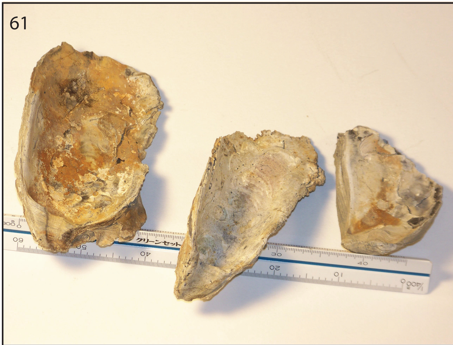
Fig. B1.2: Photograph of shells from grab #61 before selection of shell to date from a grab, and prior to cutting of shell subsample to be dated. Shells have been rinsed and dried, but have not been vigorously cleaned yet. Shell on the left hand side was selected and cleaned prior to cutting.
