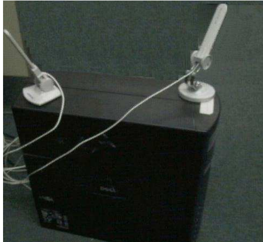
Figure 6.2: A Hyacinth mesh node built using standard Dell desktop. The two antennas are separated by 2 feet to reduce inter-NIC interference.
