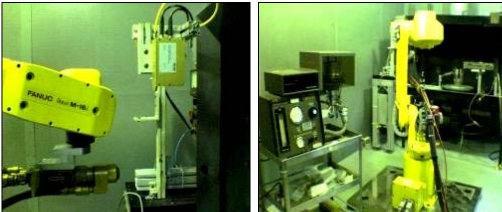
Fig. 1. Water cooled HVOF DJ-Gun 2700 at the Center for Thermal Spray Research at Stony Brook University, NY
