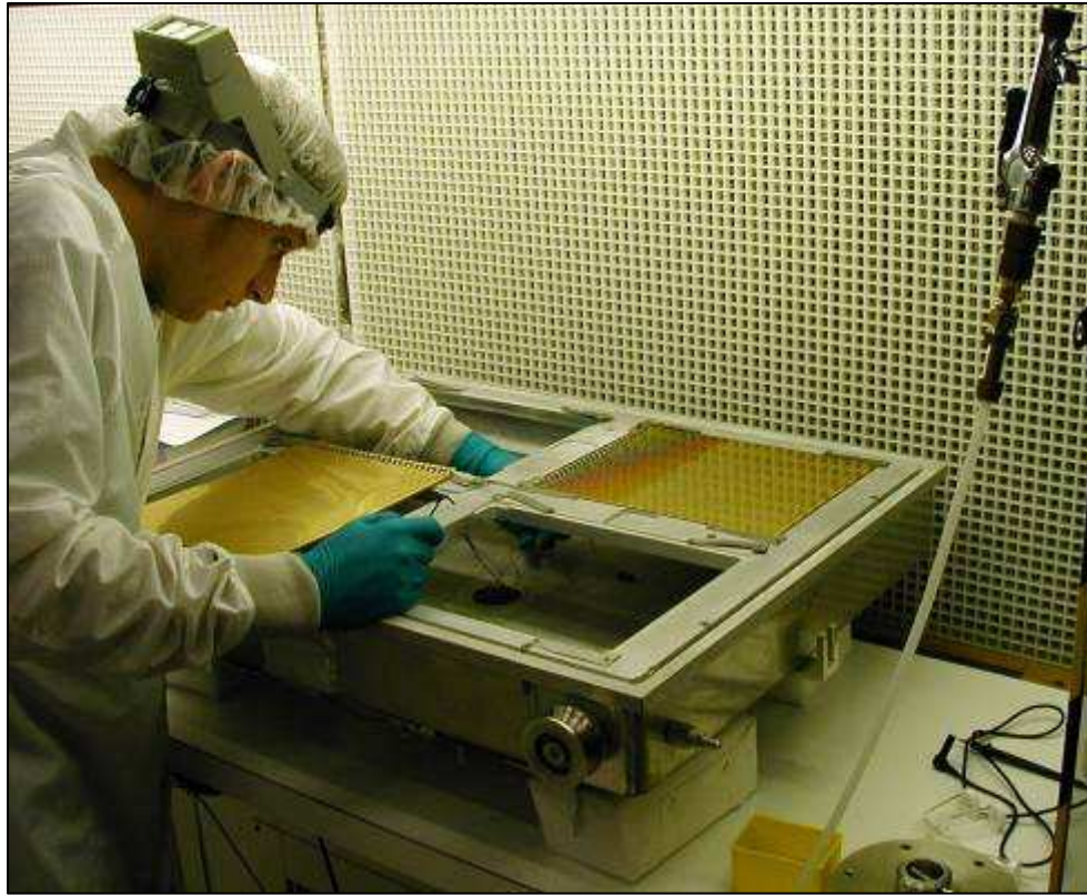
Fig. 17: Mounting the GEMs into the evaporation box.
