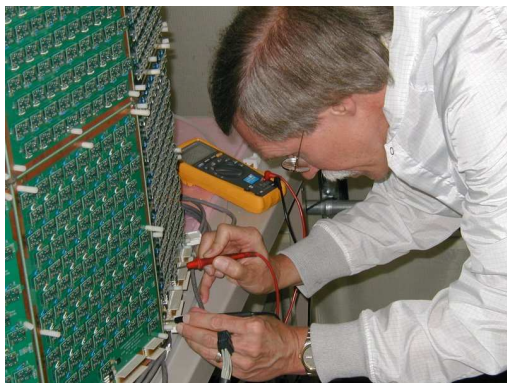
Figs. 69, 70: Voltage testing the preamplifier power components, running a battery of commissioning tests.
