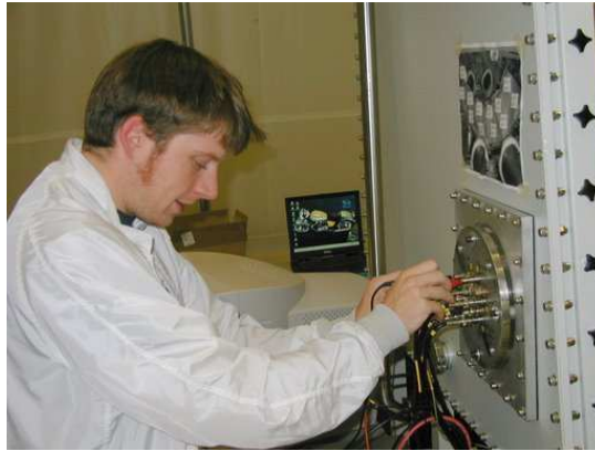
Fig. 36: Testing for continuity and capacitance.
