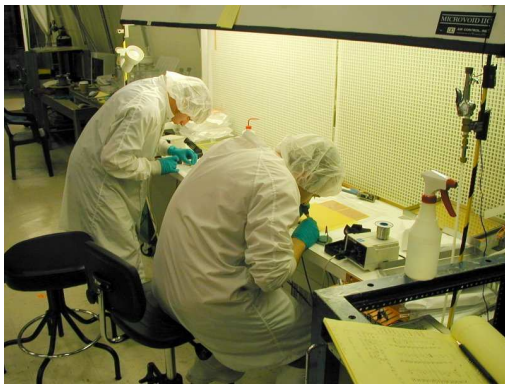
Figs. 67, 68: Repairing GEM leads on the laminar flow table, all hands at work building HBD West.
