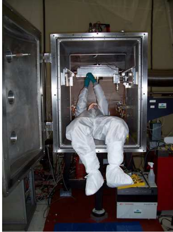
Fig. 19: Inside the evaporator, preparing for evaporation.
