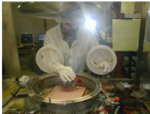
Fig. 32: Testing voltages on each strip.
