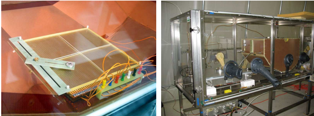
Figs. 55, 56: Single GEM stack in the prototype, prototype vessel in the old glove box.
