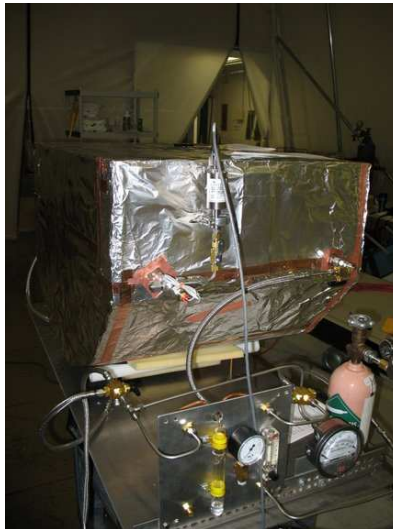
Fig. 59: Prototype HBD, under transport gas flow, awaiting shipment to BNL for Run 06.
