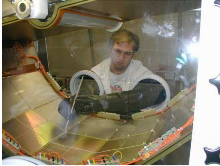
Fig. 37: Tightening down the GEMs within the vessel.
