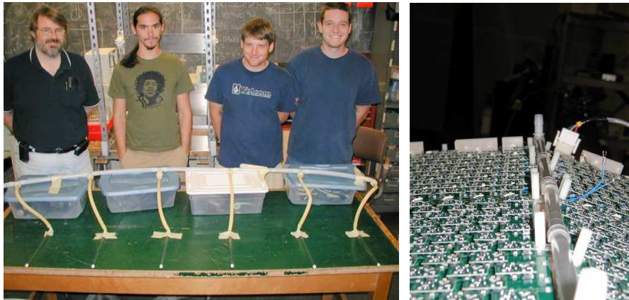
Figs. 47, 48: Prototype cooling system, and final placement in between preamplifiers.
