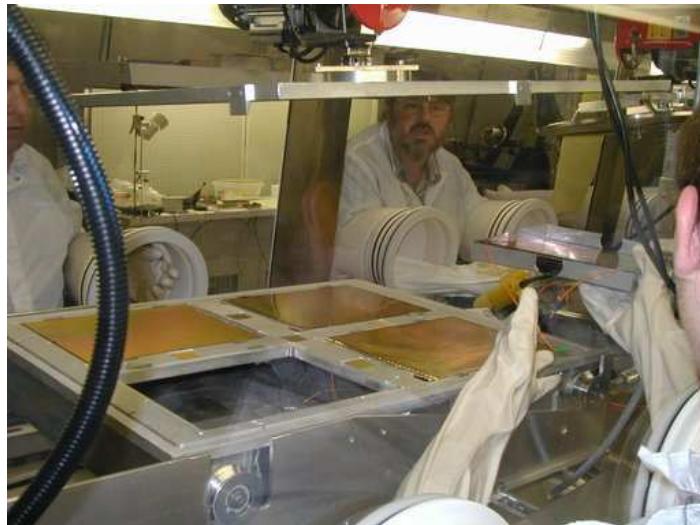
Fig. 30: Removing CsI coated GEMs from the evaporation box, while inside the glovebox.
