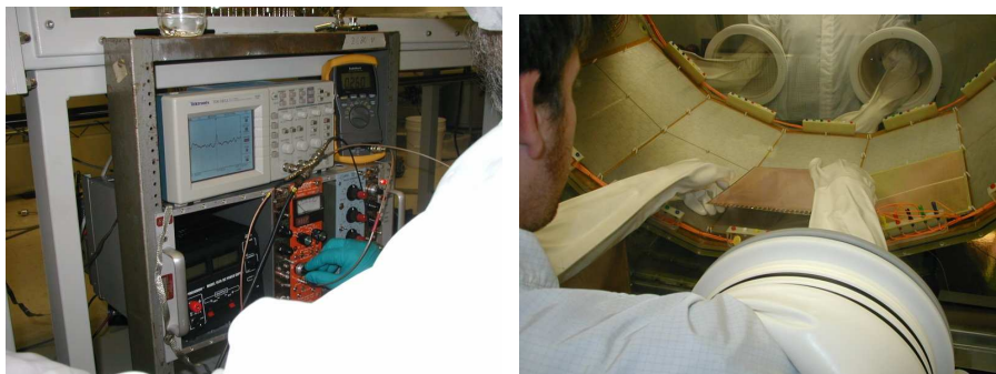
Figs. 65, 66: Running tests within the gain test station, building a tested GEM stack in the HBD.
