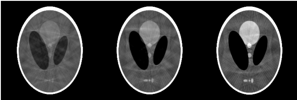
Figure 3.7: Feldkamp reconstruction from 8-bit data. Left: 0.5% contrast; Center: 1% contrast; Right: 2% contrast.
