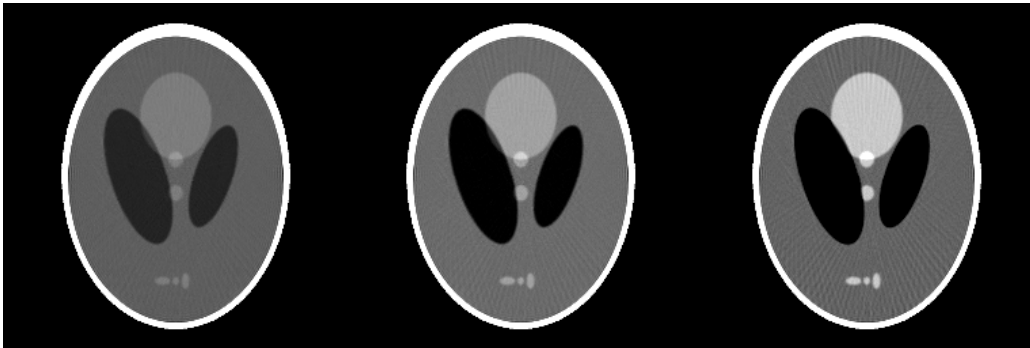
Figure 3.9: Feldkamp reconstruction from pseudo-16bit data. Left: 0.5% contrast; Center: 1% contrast; Right: 2% contrast.
