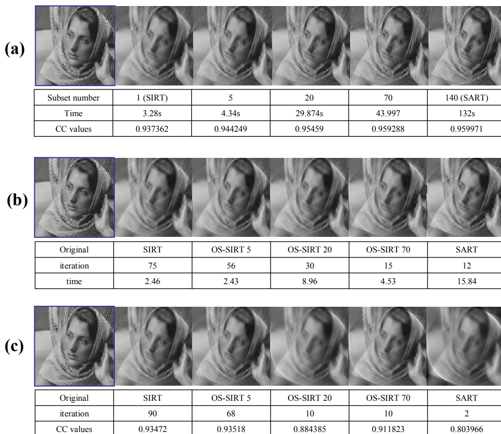
Figure 4.10: Barbara image, reconstructed via various ordered subset methods. The image resolution is 256 \times 256 all reconstructions were run from 140 projection angles. Linear interpolation was used in all reconstructions. (a) Reconstructions obtained for various numbers of subsets after 100 iterations (b) Reconstructions obtained for various numbers of subsets for a fixed CC = 0.93. We observe that the best result is achieved for 10 subsets. (c) Reconstructions obtained for various numbers of subsets for a fixed time = 2.95s. We observe that again the best result is achieved for 10 subsets.
