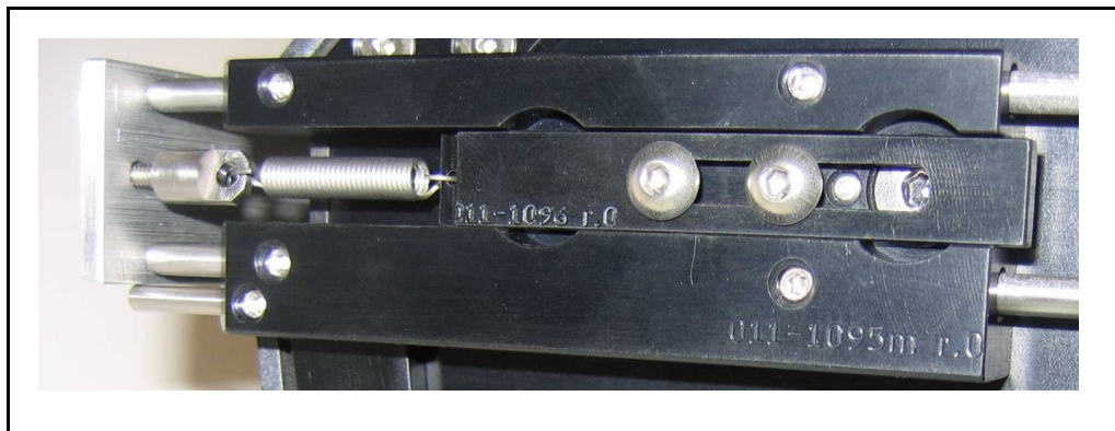
Figure 31: Knife-edge holder. The sample is held using screw-hook system and spring
