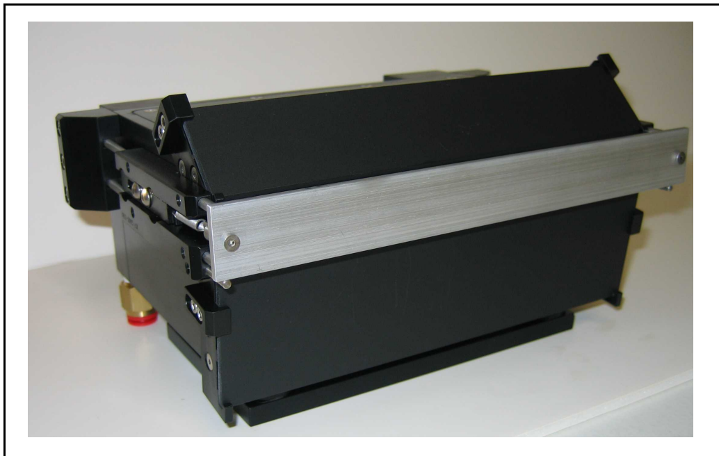
Figure 30: In-situ coating property sensor (ICP-4) with an aluminum sample mounted
