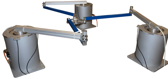
Figure 1.1: A 3-RRR planar parallel manipulator. Source: Institute of Mechatronic systems, Leibniz Universität Hannover
