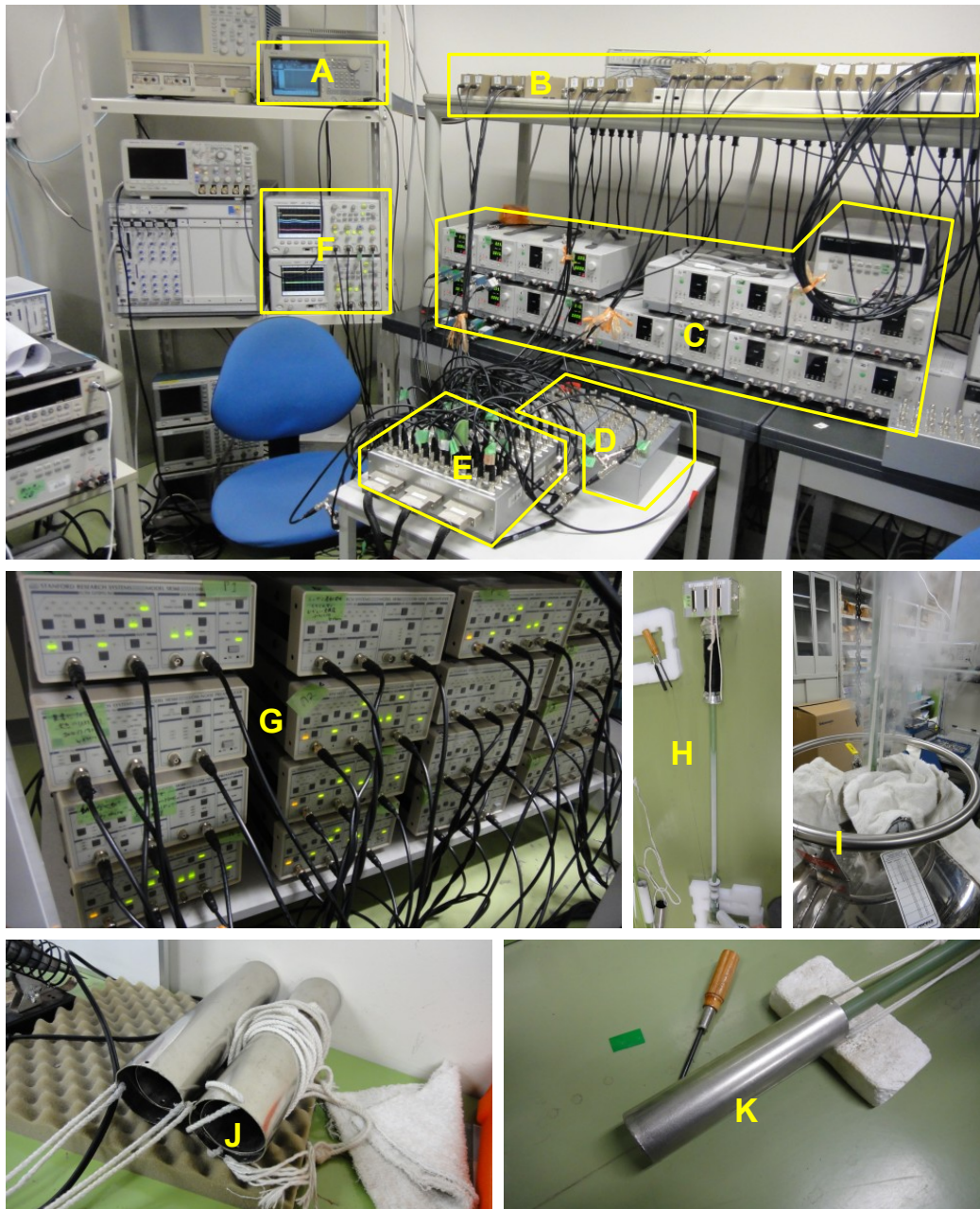
Figure 5.19: Equipment used for experimental testing: (A) data generator, (B) input attenuators, (C) power supplies, (D) low-pass filters, (E) probe connection box, (F) oscilloscopes, (G) differential amplifiers, (H) chip probe, (I) Helium Dewar with chip probe inserted, (J) magnetic shields, and (K) magnetic shields attached to chip probe.
