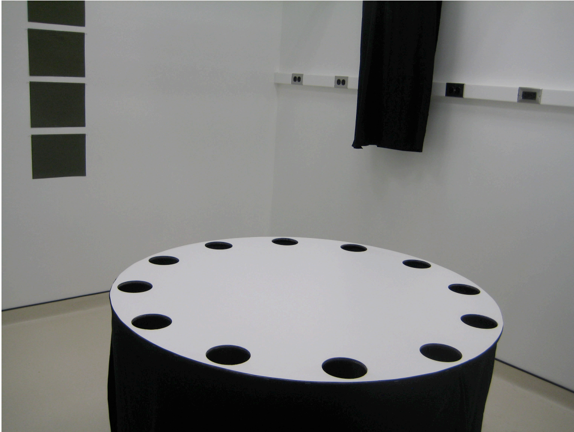
Figure 3: Barnes Maze used for Behavioral Testing. Maze dimension include a four feet diameter with twelve evenly spaced holes surrounding the periphery – one of which leads to a recessed goal chamber. Logitech Carl Zeiss HD1080P video camera hung directly above the platform to record all behavioral trials.
