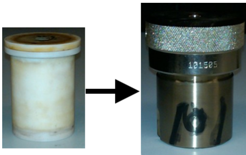
Figure 2.1. The Teflon liner (left) and Parr autoclave (right) in which the liner is sealed.
