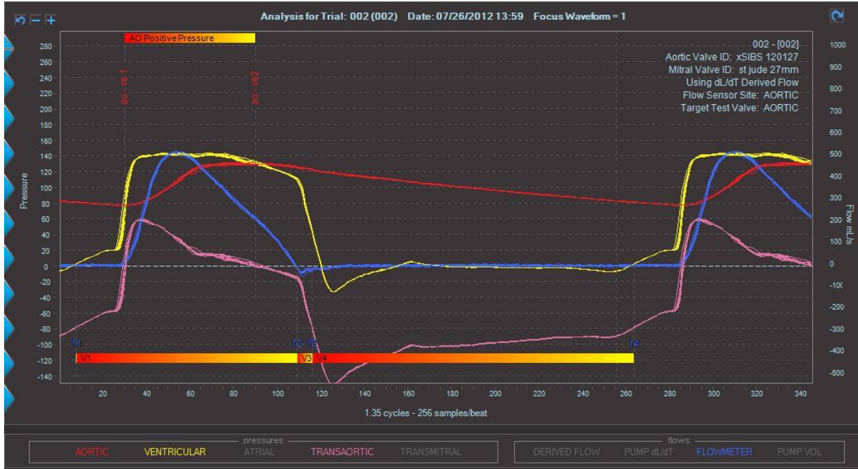
Figure 40: Representative graphical output from Vivitest; xSIBS valve test data shown.
