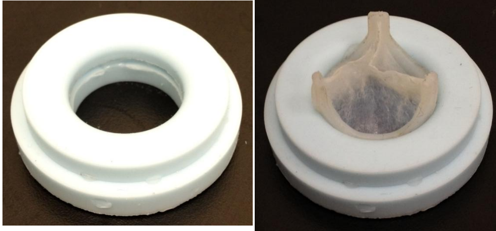
Figure 39: LHS molded silicone rubber valve holder (left, notice suture ring groove on the inner surface) with xSIBS optimized valve (right).
