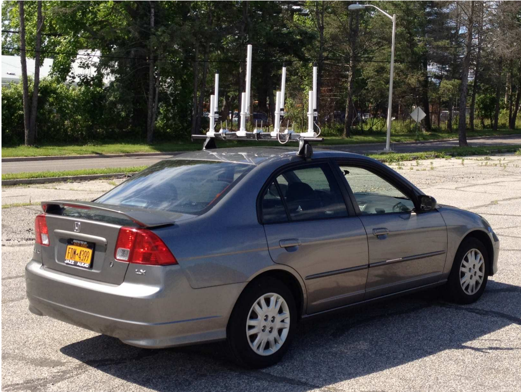
Figure 49: Picture of vehicular antenna setup used for the driving experiments.
