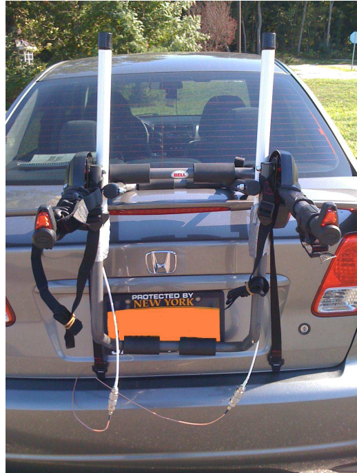
Figure 27: Two 8 dBi omni-directional antennas are mounted at the back of the car using a bicycle rack.
