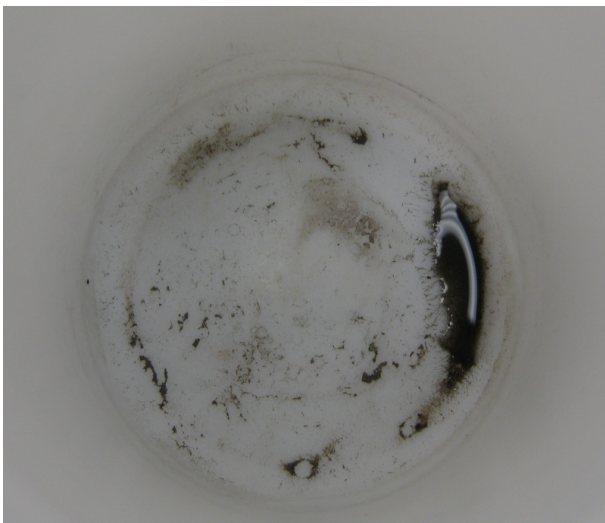
Figure 6.3: (top left) Digestion set-up both pure dust and filter samples placed in acid-washed Teflon beakers covered with Teflon eye glasses. (top right) Pure dust sample in aqua regia digestion phase. (bottom left) Pure dust sample after dry down, black carbon shown as residual. (bottom right) Teflon filter after acid digestion before final rinse.
