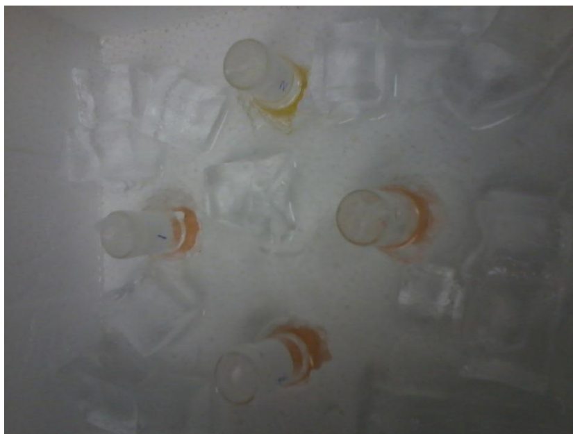
Figure 4- 1 Low temperature condition for growing crystal
