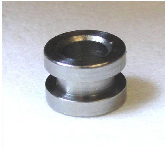
Figure 3.6: Nickel Prototype Cathode An actual nickel prototype cathode with a groove and ID.
