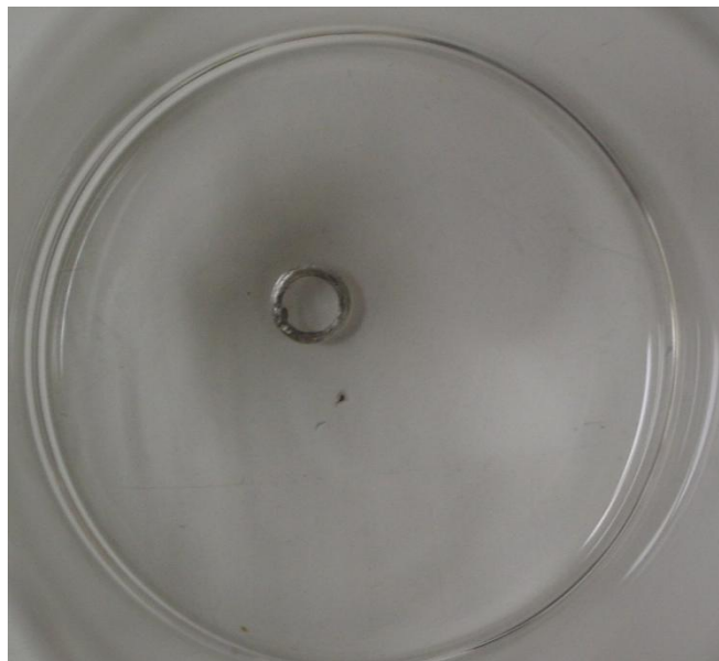
Figure 3.12: Indium Etching An example of an indium ring during the etching process.
