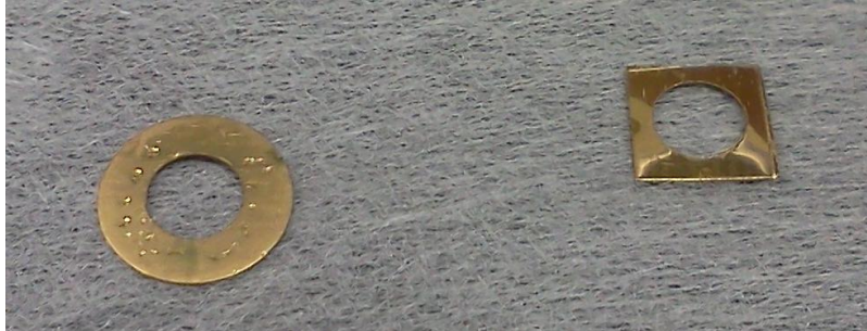
Figure 4.4: AuSi Ring and Square An example of an AuSi ring (left) and AuSi square (right).
