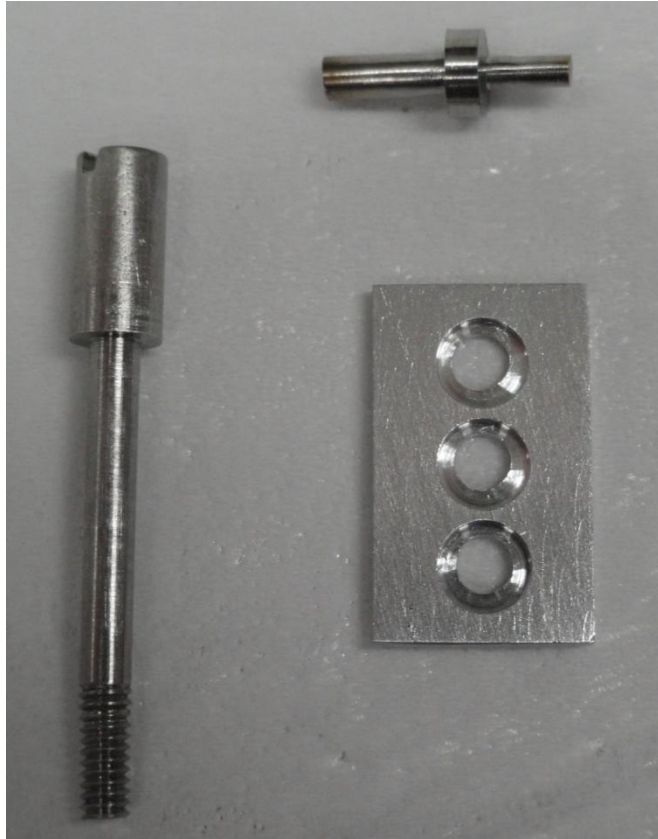
Figure 4.19: Pin, Plunger, and Plate Examples of a pin (left), plunger (top), and plate (right) that are used in the spring lock mechanism.
