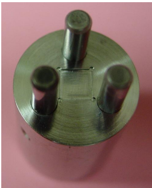
Figure 3.20: Square Recess Sample Holder The holder in which the samples were stacked. The three pegs were used for centering, along with the square recess for the diamond.
