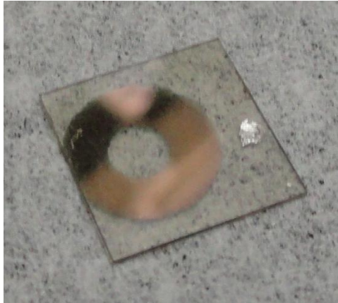
Figure 4.13: Sputtered GaN A picture of the GaN after sputtering. The sputtered ring is off center in order to choose a pristine GaN surface.
