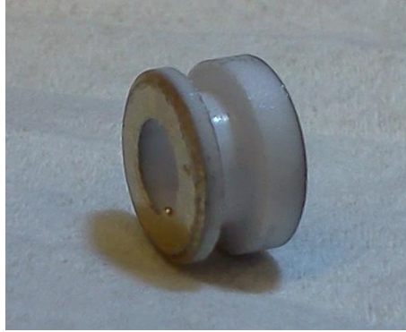
Figure 4.1: Grooved Metalized Alumina An example of the grooved metalized alumina.
