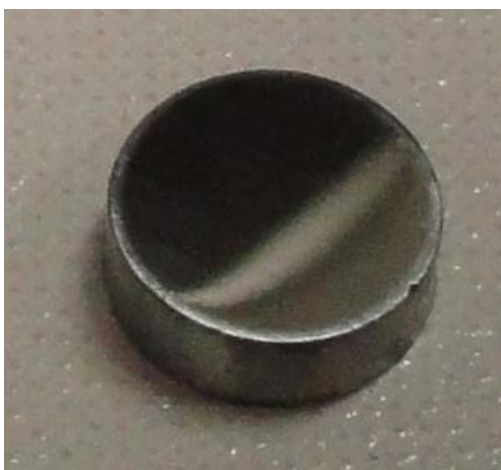
Figure 3.4: Nickel Cathode An example of a polished nickel cathode with 6 mm OD and 2 mm thickness.
