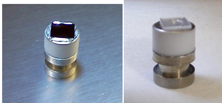
Figure 3.25 (left): Low Quality Diamond Prototype Capsule A complete indium cold welded prototype capsule with a black diamond. Figure 3.26 (right): Higher Quality Diamond Prototype Capsule A representation of what a complete indium cold welded prototype capsule with a higher quality diamond would appear as.
