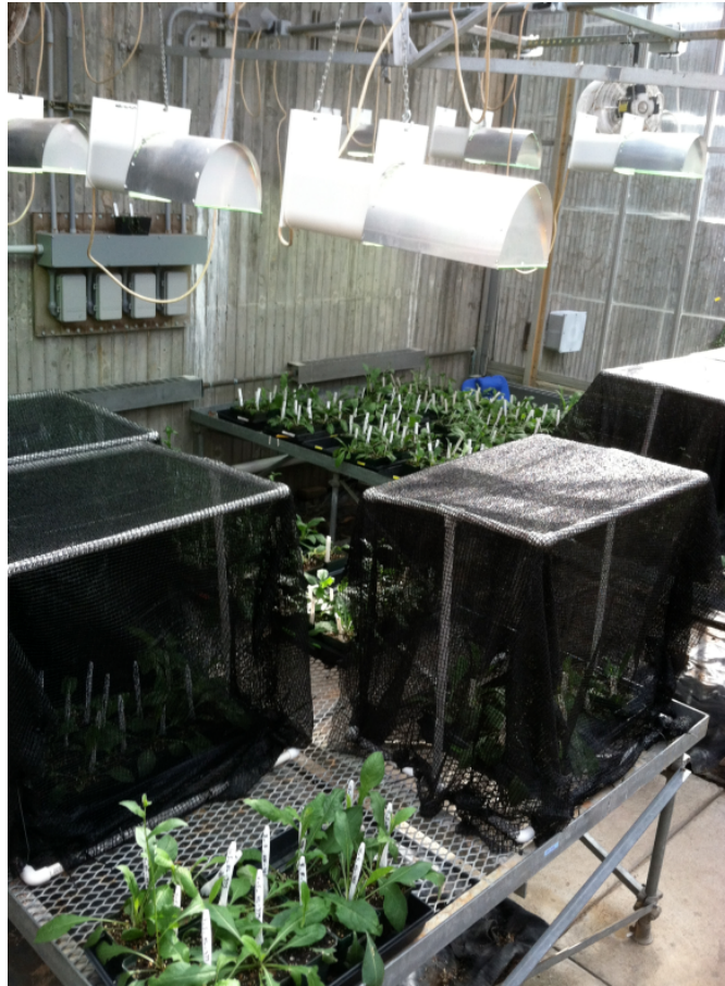
Figure 1. Shade boxes constructed for low light treatment from ¼ inch PVC and covered with 50% shade cloth.
