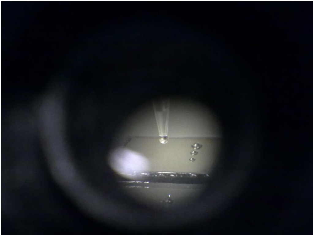
Figure 4. View through microscope of drop being deposited onto surface. Three drops on Si substrate and one falling drop can be observed through the microscope.
