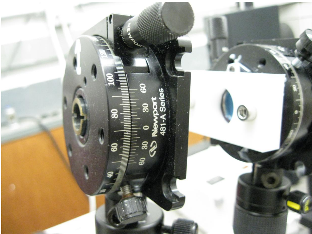
Figure 9. Rotate the polarizer to make the 71.67^\circ scale line aligned with the zero-scale line. Next, we need to determine the relation between the polarization angle and the angle of half-wave plate. We place a linear polarization after the half-wave plate, aligned with the sample \hat{y}_{\text{sample}} direction. We call this “horizontal” polarization. Light polarized 90^\circ with
