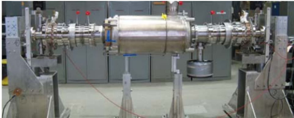
Figure 3.2: The ERL cavity string.
