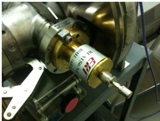
Figure 4.17: Mock FPC inserted into gun cavity. In this case, a 50-Ohm termination is attached to the FPC.
