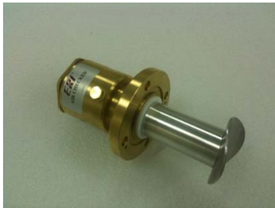
Figure 4.16: Mock FPC probe showing coupler with inner conductor and "pringle" tip attached.
