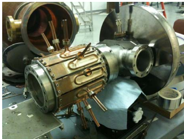
Figure 5.11: Niobium cavity with ceramic/ferrite damper attached. Note the pickup probe, attached to the RF pickup right of center. For measurements, all of the openings including the beampipe and the FPC ports were covered by shorting plates.
