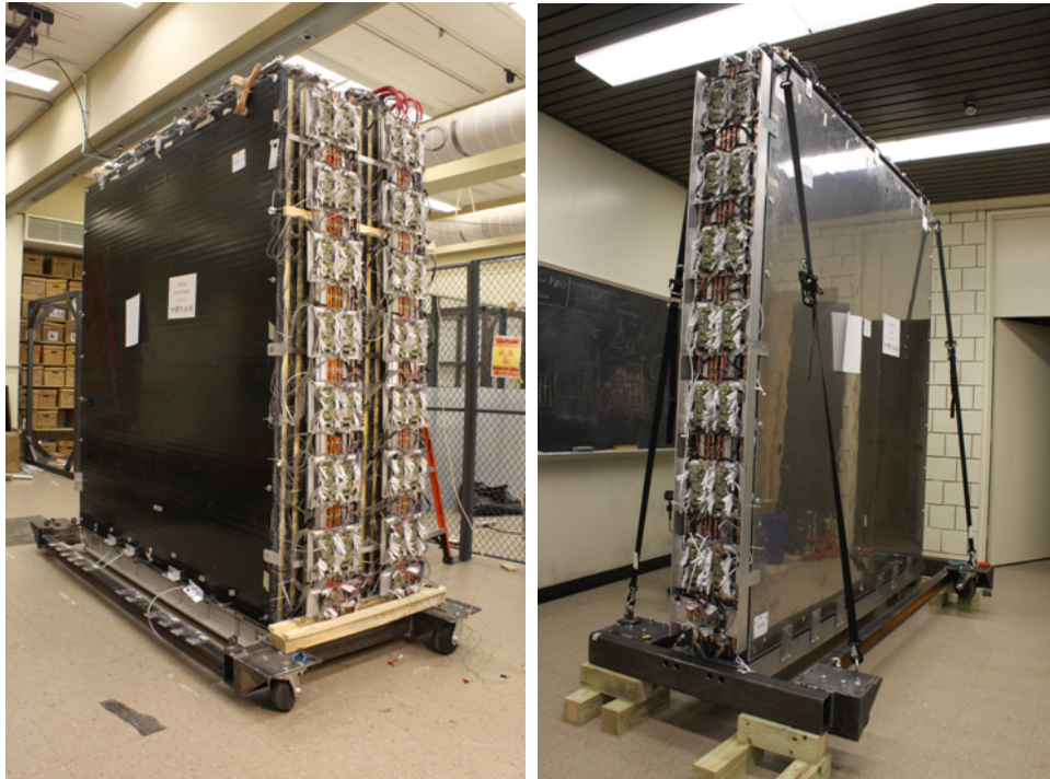
Figure 3.5: Completed Super-P0Dules. Left: The central water target Super-P0Dule. Right: The central ECal Super-P0Dule.
