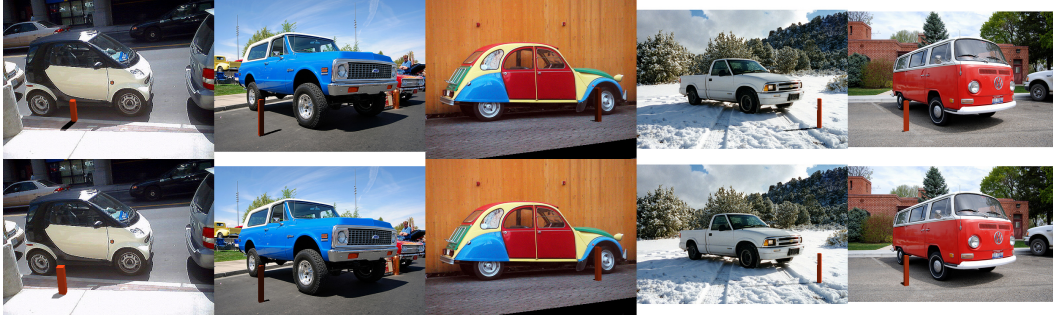
Figure 5.5: Results with images of cars from Flickr. The results of illumination estimation are presented by rendering a synthetic orange sundial to the original image, using the estimated illumination. Top: the results with our method; bottom: results with the much more computationally intensive method proposed in [129]. Our results are equivalent or better than the results from [129], although our method uses only simple shadow edge detection and a much more efficient optimization to estimate illumination parameters.
