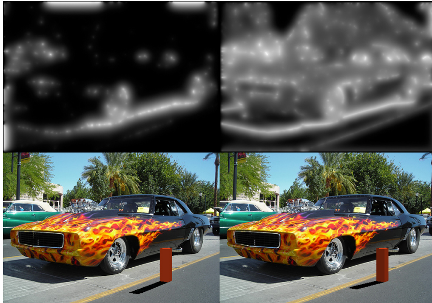
Figure 5.7: Results comparing illumination estimation based on potential shadow edges (left) and all edges in the image (right). It is clear that our method can work even when we do not explicitly detect shadow edges, because few image edges match potential shadow silhouettes. The results of illumination estimation are presented in the bottom by rendering a synthetic orange sundial to the original image, using the estimated illumination. Maps Q are in the top row. This is an image where we failed to obtain any meaningful illumination estimate with the method of [129].
