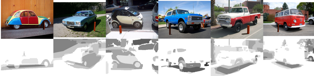
Figure 6.8: Results with car images collected from Flickr. Top row: the original image and a synthetic sun dial rendered with the estimated illumination; Bottom row: the final shadow labels. The geometry consists of the ground plane and a single bounding box for the car.
