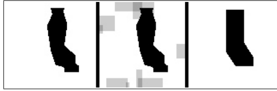
Figure 5.3: Examples of synthetic images used for quantitative evaluation. Image size was 100x100 pixels. From left to right: a) the full-resolution 3D model, rendered with 1 point light source; b) the full-resolution 3D model, after the addition of noise, as described in the text (noise is random and may coincide with the shadow); c) the approximate 3D model corresponding to the full-resolution model on the left, rendered under the same illumination (for demonstration; this model is used for the illumination estimation only, in the experiments with approximate geometry).
